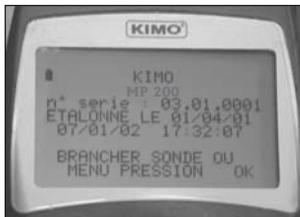
To access to the menu pressure, press on the knob ; To access to another menu, connect the corresponding probe. If this one uses the SMART PRO system, the screen shows the type of the connected probe, and its calibration or adjusting date. To access to the menu press on the knob. To return to the homepage, disconnect the probe or press on "ESC" for the menu pressure.
